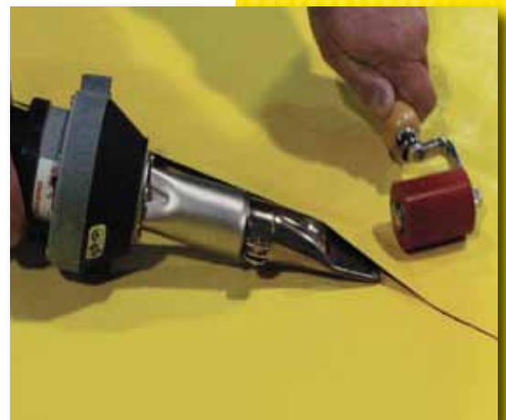
Hand Detail Welding
