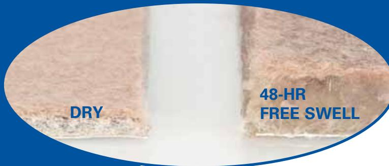
Upon hydration, the APC core expands to form a dense, impervious waterproofing membrane.
