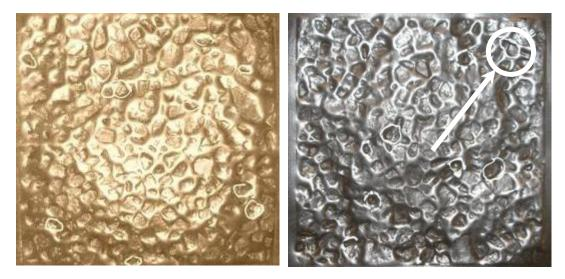
Figure 1. Comparison of 60-mil (1.5 mm) LLDPE Geomembrane tested in contact with 1/2" to 1" (12 to 25 mm) rock at 585 psi (4033 kPa) for 48 hours, both with (left) and without (right) underlying GCL.
